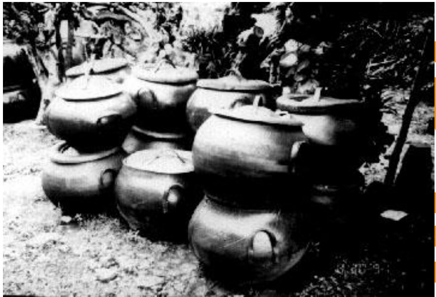
Figure 4: Garbage containers made from Truck tyres. Manila, The Philippines. Photo: CAPS - WASTE
